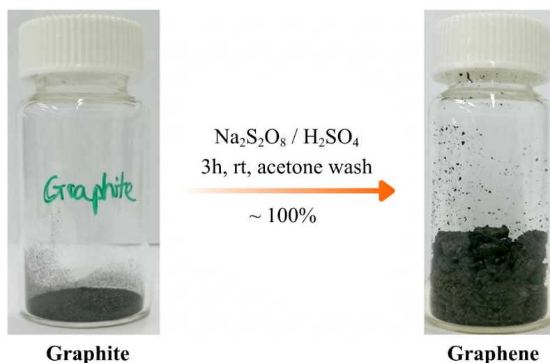
Figure 3. Synthetic route of the graphene nanoplatelets from natural graphite. Reproduced from (La et al. , 2016) with permission from Wiley
