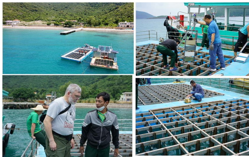
Figure 1. Installation of plates with experimental coatings at the Marine Research and Testing Station (MRTS) “Dam Bay,” located on the Island in Dam Bay Gulf (12°14' N, 109°11' E). Approximate distance from the sea: 100 meters
